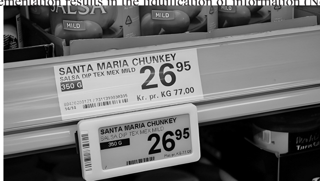
Figure 1 ESL, Lower One, Attached to the Front Edge of Retail Shelves Note: Source: e-Ink.
